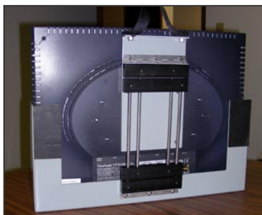
Monitor folds into the stand's base for secure storage and transport
